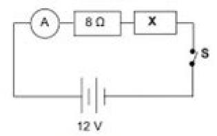
The 12 V battery has negligible internal resistance. When switch S is closed, the reading on the ammeter is 0,5 A.
