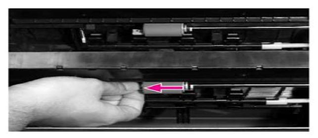
Figure 6-45 Removing the Paper Feed Rollers (HP LaserJet 4000 T/4000 TN and 4050 T/4050 TN shown)
